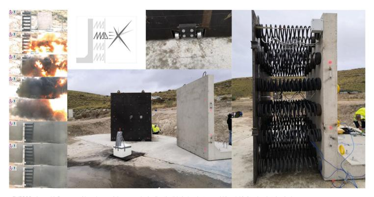
FHECOR, along with Ruesma and Inge, is one of the companies leading the 'Madex' project, an ambitious initiative aimed at developing an explosion damping wall. Field tests were conducted last November.
